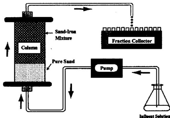
FIGURE 1. Schematic diagram of column experiment setup.
